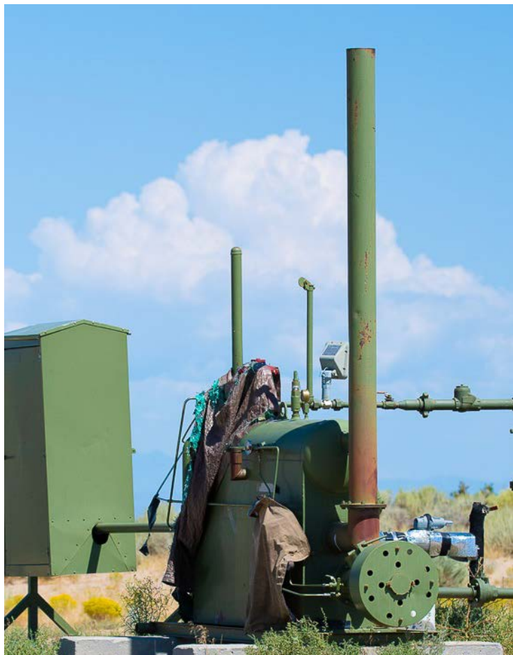
Uncovered burner/vent stacks have been responsible for numerous bird and bat mortalities. All burner/vent stacks should be covered. Photo: James Ramakka
