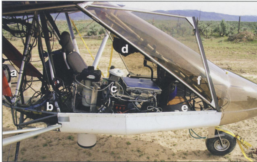
Figure 1. Sport aircraft at a Nevada site with remote sensing equipment as used over the Central Plains Experimental Range in Colorado. (a) Ballistic parachute capable of safely landing the entire aircraft in an emergency; (b) 12V battery and AC/DC inverter for powering camera, laser altimeter, and laptops; (c) aluminum equipment module supporting the Canon 1Ds digital camera and 840-mm lens, Trackair navigation box, light meter, laser rangefinder used as an altimeter, 24V power supply for Trackair system, trackball mouse and laptop computer for displaying laser-measured altitude and storing digital images; (d) LCD monitor; (e) navigation laptop computer; and (f) global positioning system receiver.
