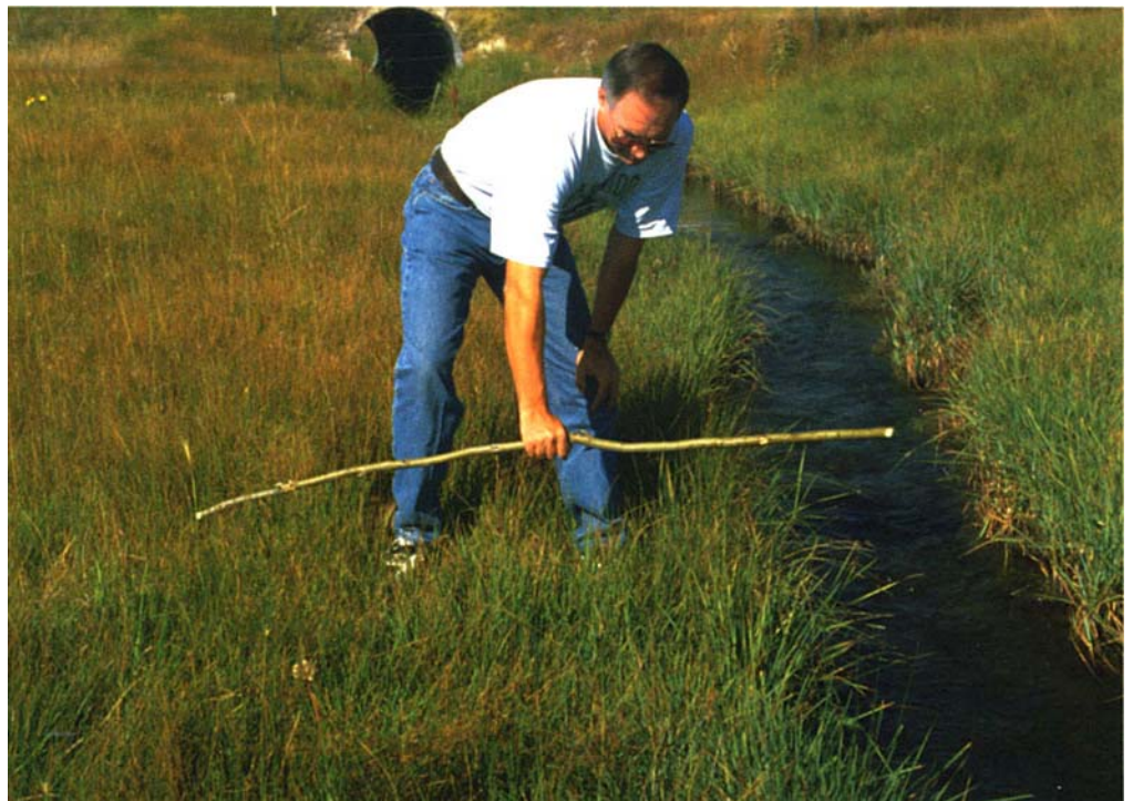
Figure 17 —Placement of the measuring pole such that the left end does not reach beyond the center of a stream less than 6 feet wide.
