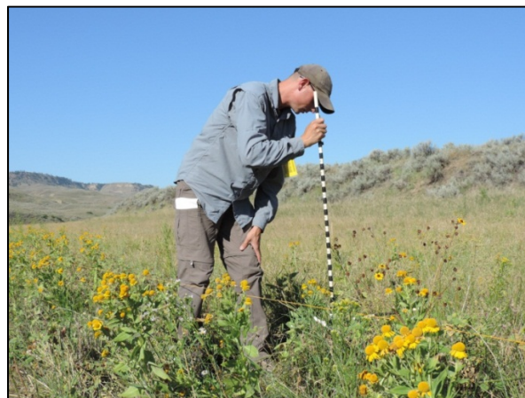
Figure 9. Using the frame handle to guide the plot directly under the tag line (T2 & T3).
