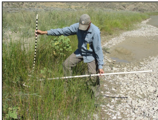
Figure 8. Using the 2-m rod to locate the plot on T1 (1m from the scour line).
