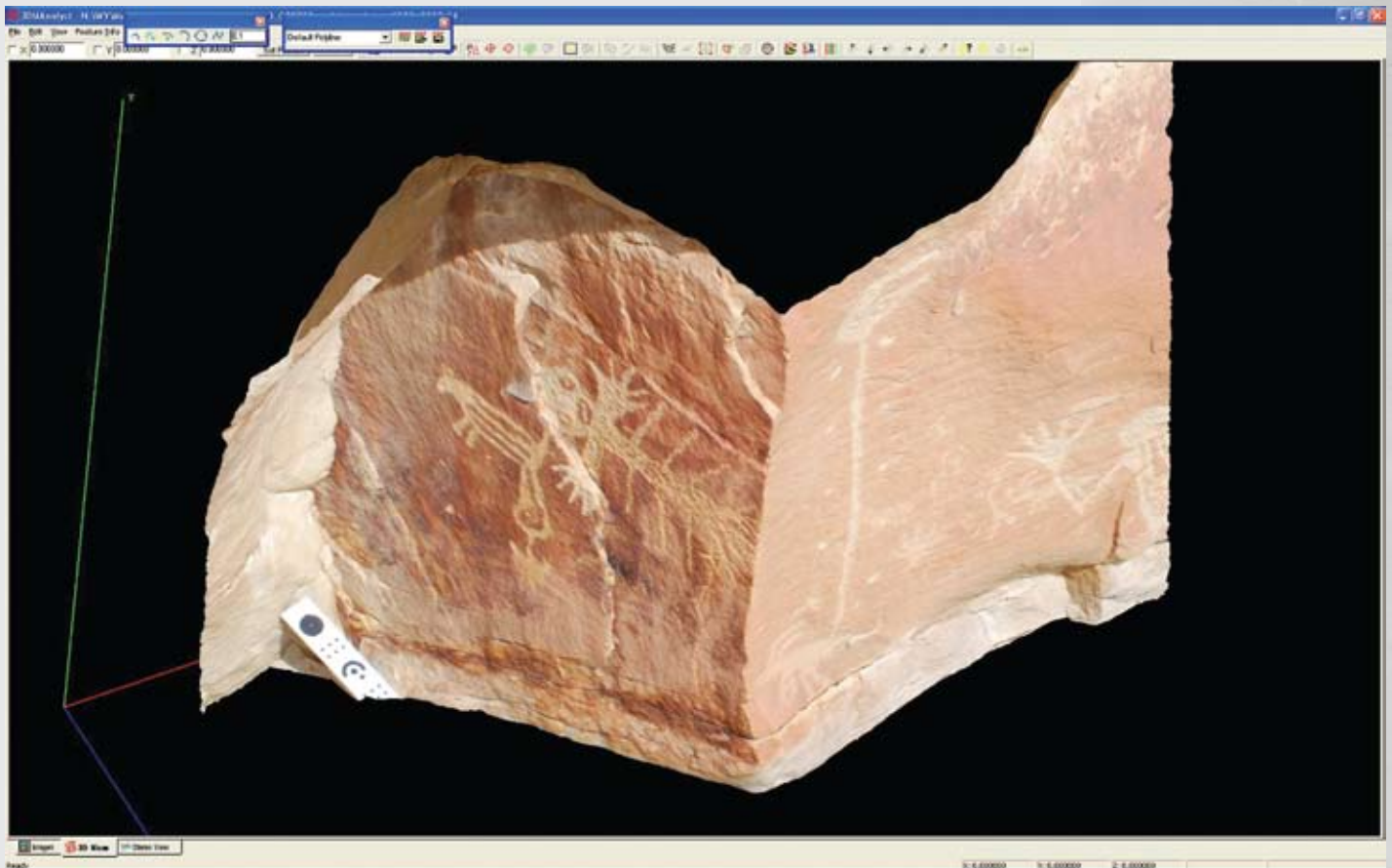
Figure 8. Three-dimensional surface and image datasets can be packaged as industry standard files that can be viewed and rotated in 3D by a number of software programs. Shown is a right angle cliff face from the Bighorn Basin, Wyoming.
