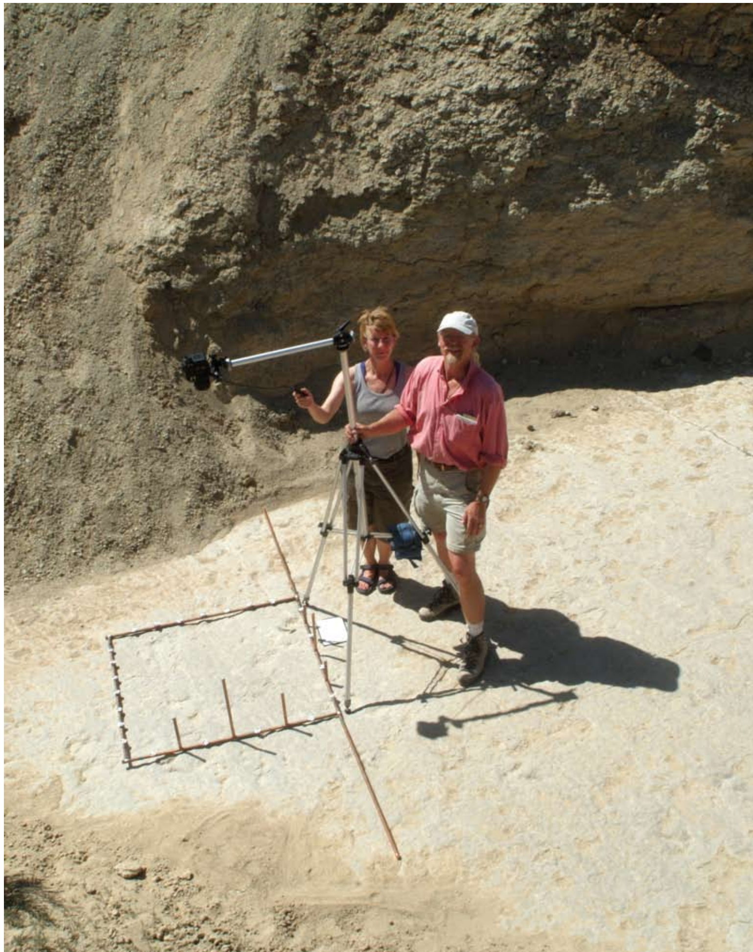
A fixed grid of varying height was used as an early method of providing x,y, and z control at the Red Gulch Dinosaur Tracksite in Wyoming.
